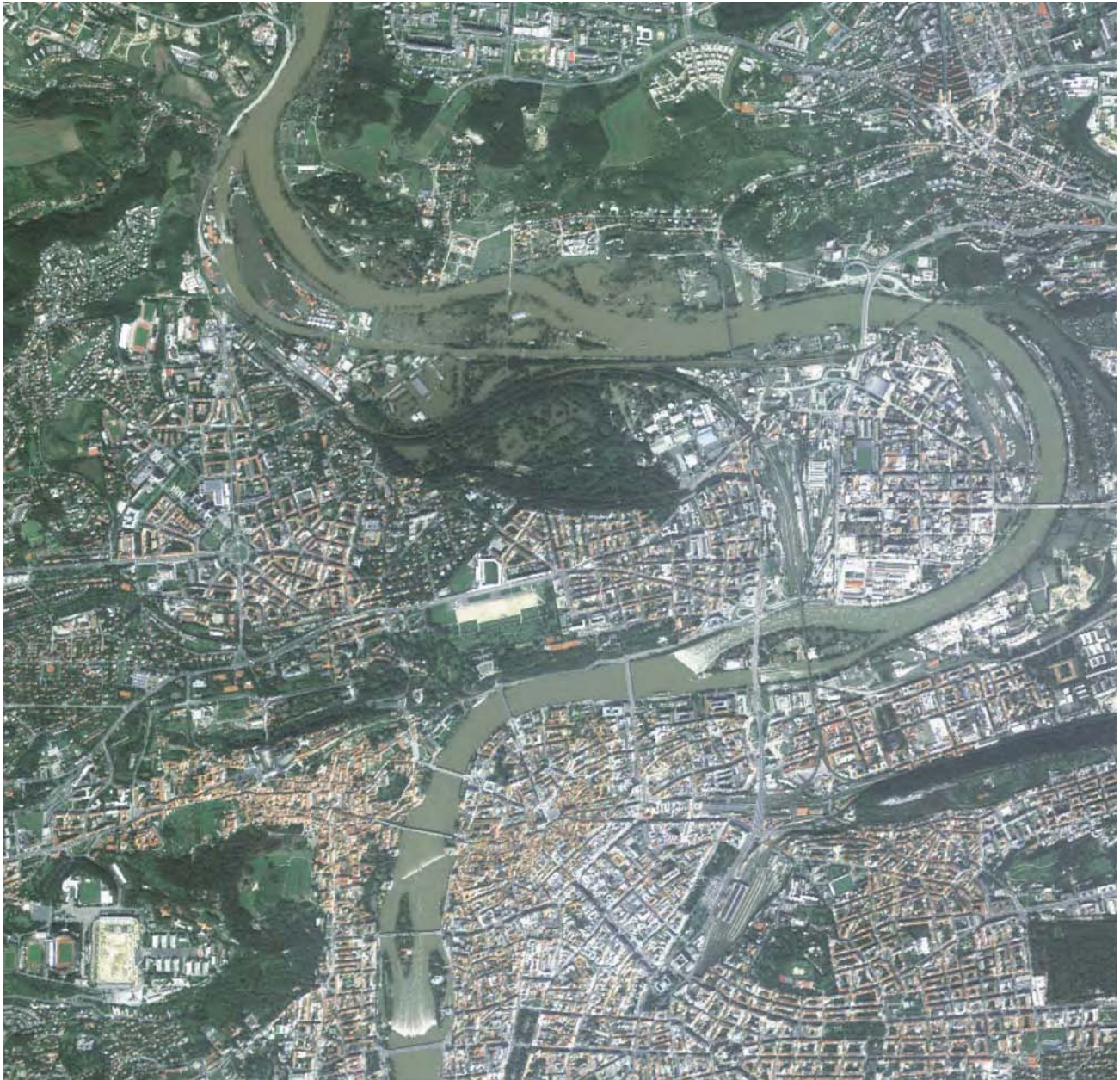
FIGURE 4 Panchromatic/multispectral merged image of Prague Czechoslovakia with effective resolution of 61 cm. (Courtesy DigitalGlobe.)
