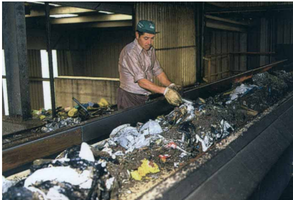
Fig. 2.6a Separation of metals on a belt in a selection plant (Revista Sostenible).
