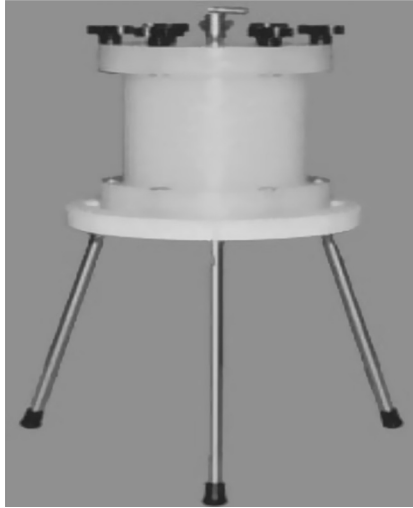
Figure 5.1 Pressure filtration unit (for the initial solid/liquid phase separation).
