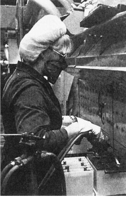
Figure 20-2. Adequate control of lead exposure for all workers requires a high level of engineering control and may also require personal protective equipment. Because U.S. law prohibits exclusion of pregnant women from lead work, controls must be sufficient to protect the fetus as well. (Source: Saryan LA, Zenz C. Lead and its compounds. In: Occupational medicine (3rd edition). Zenz C, Dickerson OB, Horvath EP, Jr. St. Louis: Mosby Year Book, Inc., 1994, p. 507. Reproduced with permission.)
