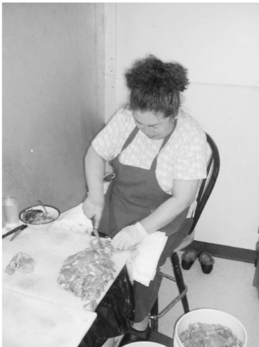
Figure 16-2. Woman in Nicaragua cutting meat. A high degree of hand force and frequent repetition combine to make this a high-risk job for development of carpal tunnel syndrome and tendonitis. In addition, this woman faces the potential hazards of cuts and neck strain. (Photograph by Barbara Silverstein.)
