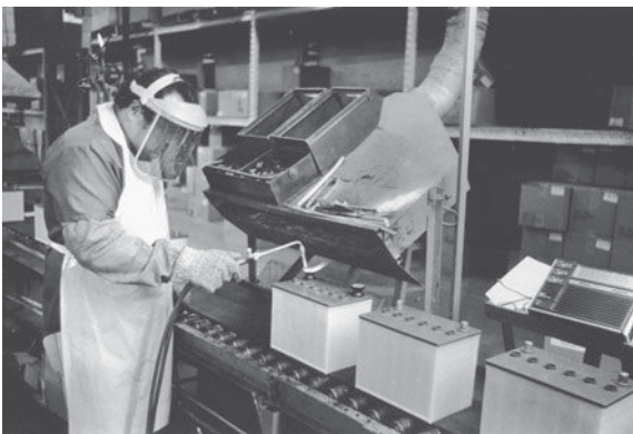
Figure 19-2. Current work practice rules require significant personal and environmental protection in situations of lead exposure: (A) Lead battery worker is protected mainly by local exhaust ventilation. (B) Automobile lead grinder is protected by air-supplied hood and floor exhaust ventilation. (Photographs by Earl Dotter.)
