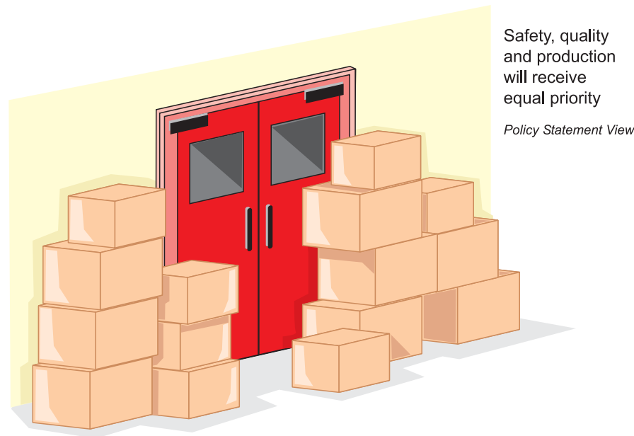
Figure 2.4 Sound policy but not put into practice – blocked fire exit.
