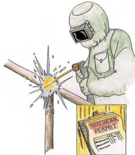
Figure 6.10 Hot work permit is usually essential except in designated areas.
