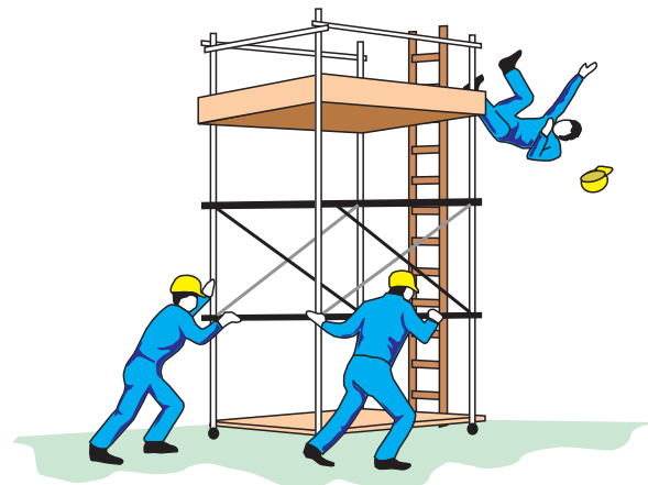
Figure 7.3 Falling from a height – tower scaffold.
