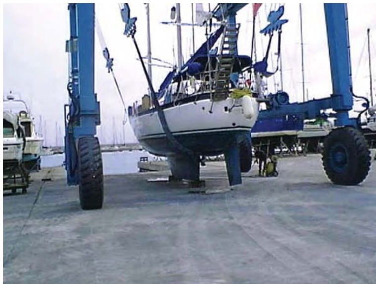
Figure 8.11 Manoeuvring a yacht using a large overhead travelling gantry and slings in a marina.
