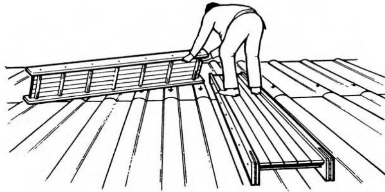
Figure 14.2 Proper precautions must always be taken when working on or near fragile roofs.
