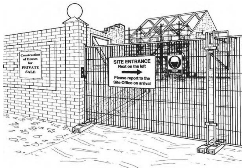
Figure 14.1 Secure site access gate.
