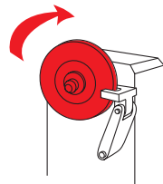
Abrasion and Ejection Hazard
