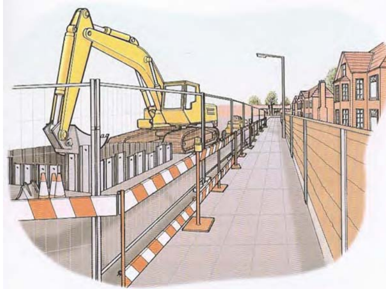
Figure 14.3 Barriers around excavation by footpath.
