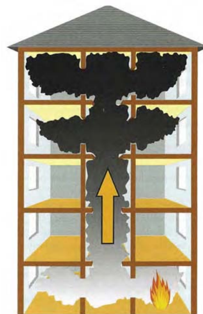
Figure 11.4 Fire spread in buildings.
