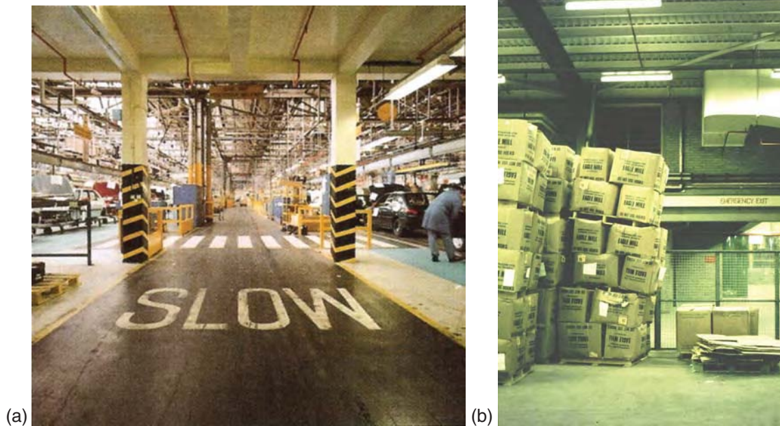
Figure 7.5 (a) Internal roadway with appropriate markings; (b) unsafe stacks of heavy boxes.
