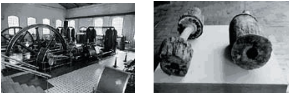
Figure 26.5 Exposition Museum of Riga Water Supply in Baltezers with steam pumps and remnants of wooden pipes used in the 17 th century (Source: Archive materials of Riga Water Ltd.)
