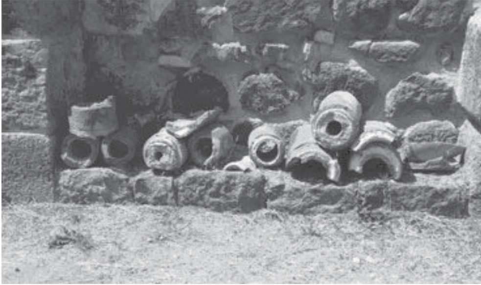
Figure 5.7 Various degrees of calcium carbonate incrustation seen in sections of Roman water pipes piled up against the wall of a Roman bath in the town of Kos, island of Kos, Greece. (Photo: Marjatta Vuorinen)
